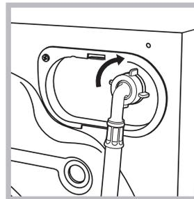
2. Connect the inlet hose to the Washer-dryer by screwing it onto the corresponding water inlet of the appliance, which is situated on the top right-hand side of the rear part of the appliance (see figure).
